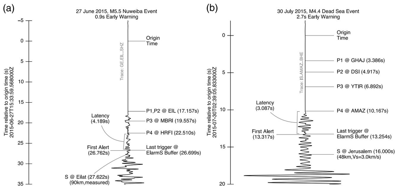
**Figure 8.** Timeline scheme for the RT processing of (a) the 27 June 2015  $M_D$  5.5 Nuweiba event and (b) the 30 July 2015  $M_D$  4.4 Dead Sea event.  $P_x$ ,  $P$ -wave arrival time at a station, in which  $x$  is the station trigger order of arrival.  $S$ ,  $S$ -wave arrival at a location.
