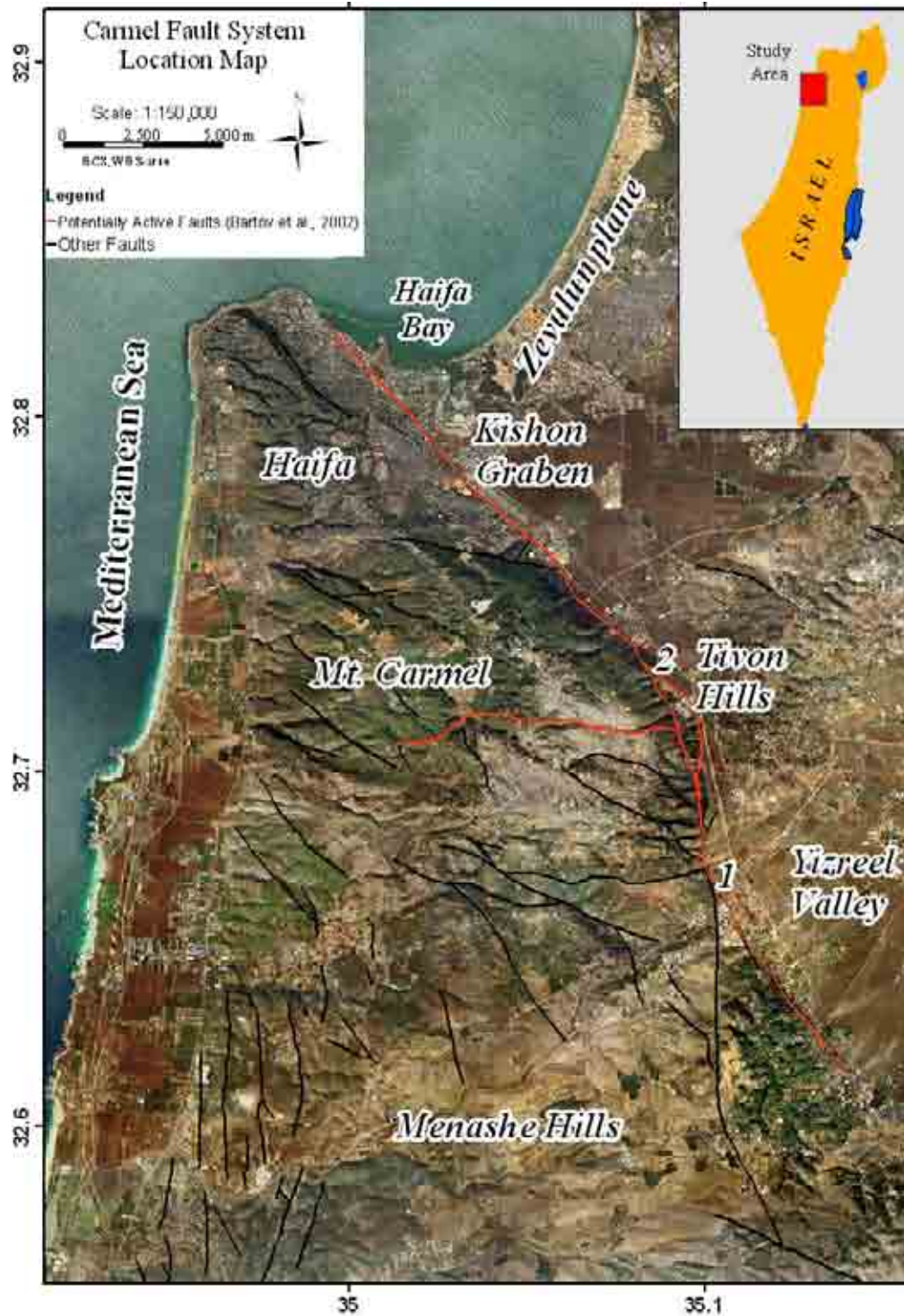
Fig 1. Location map of the Carmel Fault System (CFS) superimposed on an orthorectified aerial photograph (orthophoto). The red line marks the main fault described as a potentially active fault (after Bartov et al., 2002). Black lines are surface mapped faults (From GSI GIS database). (1) Yokneam junction. (2) Jalame' junction.
